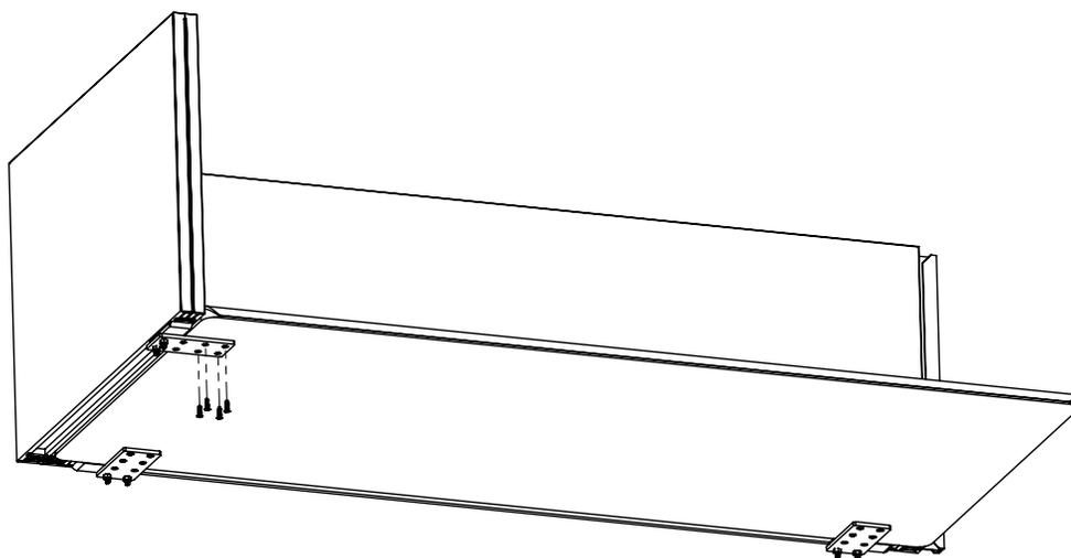
**Step 10:** Lift the privacy panel up to access the mounting bracket fasteners.
