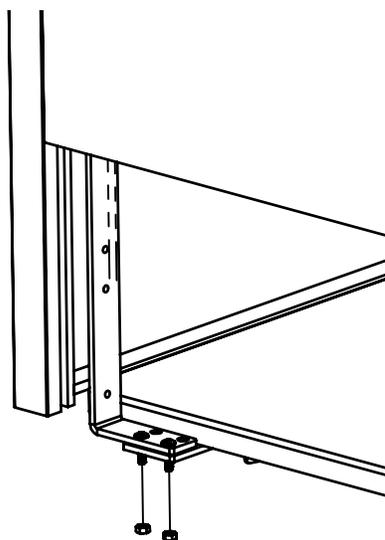
**Step 12:** Attach x2 additional mounting brackets to the exposed bolts as shown, and replace the nuts.
