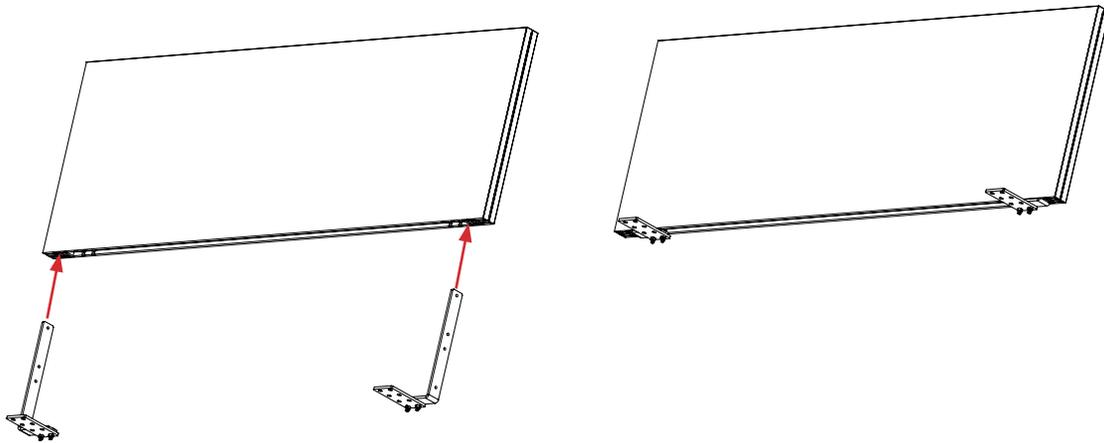
**Step 3:** Align the panel to your tabletop as shown, and screw into position with [x4] #10 wood screws per surface bracket, as shown. You may refer to the dimensions on page 05 and mount the brackets without using the panel to align, but this is the preferred method.
