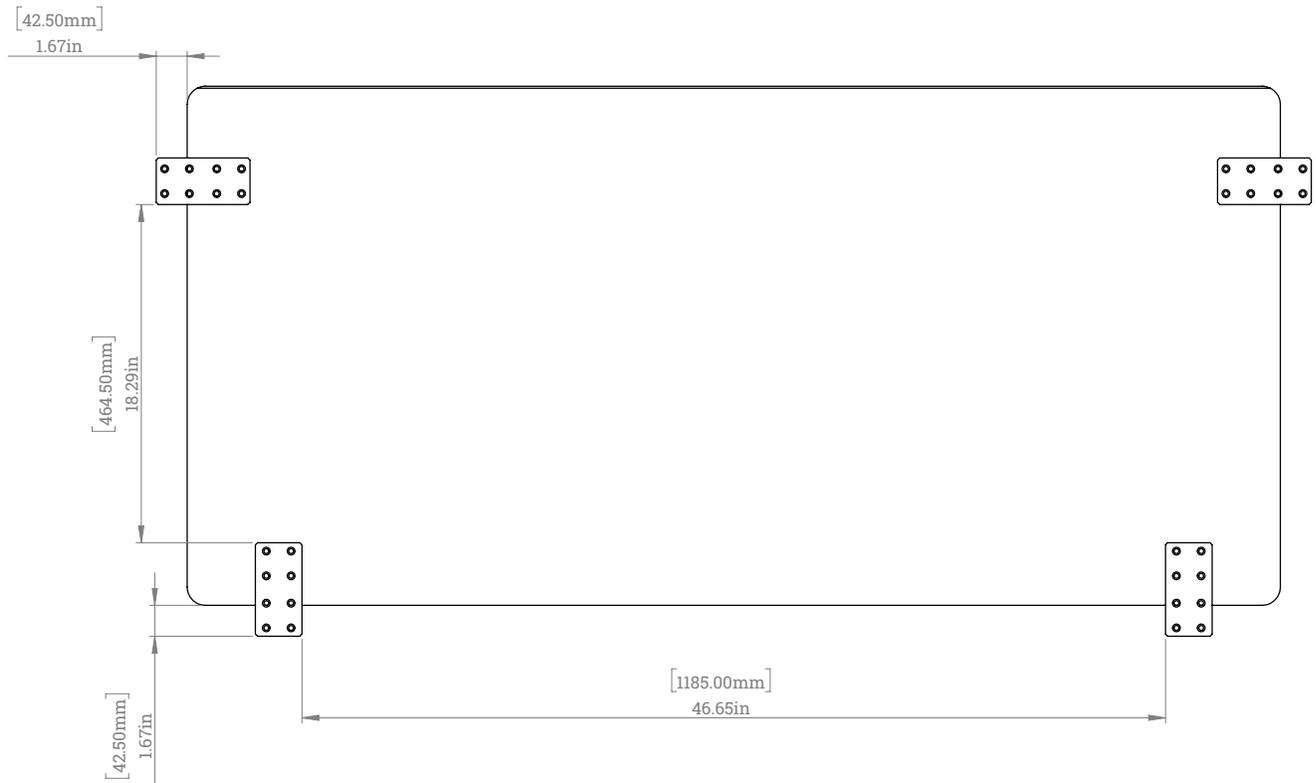
**Step 4:** Slide both 2-way connectors into the privacy panel, as shown below.
